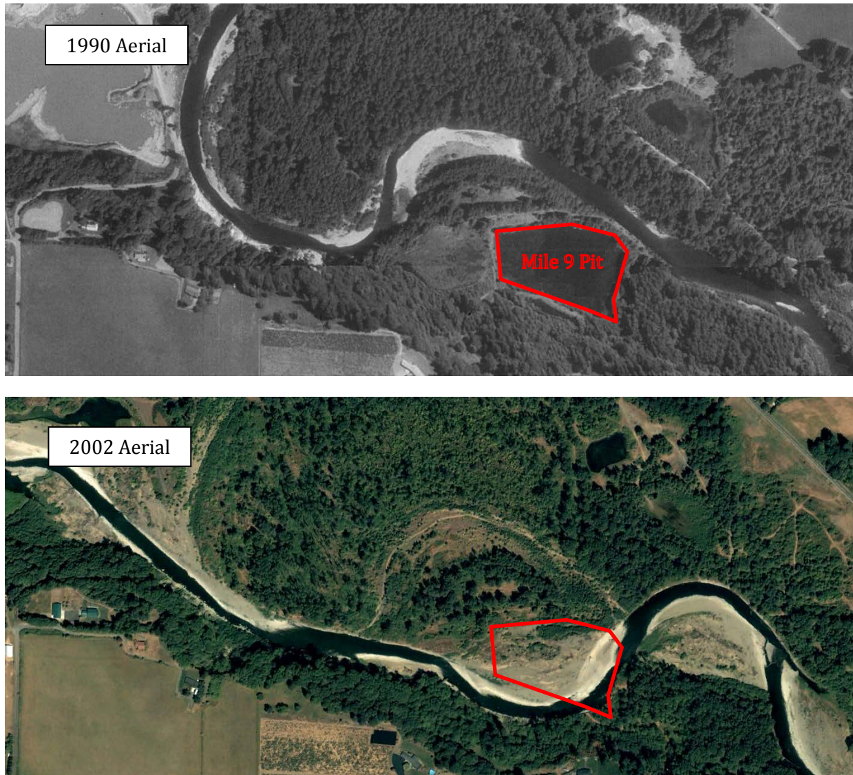
Figure 5. Location of the Mile 9 Pit avulsion, which occurred in November 1995.
