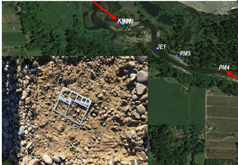
Figure 2c. Grain size analysis at selected bed sub-surface locations. Note finer materials present here, under the overlying armored surface layer with larger cobbles.
