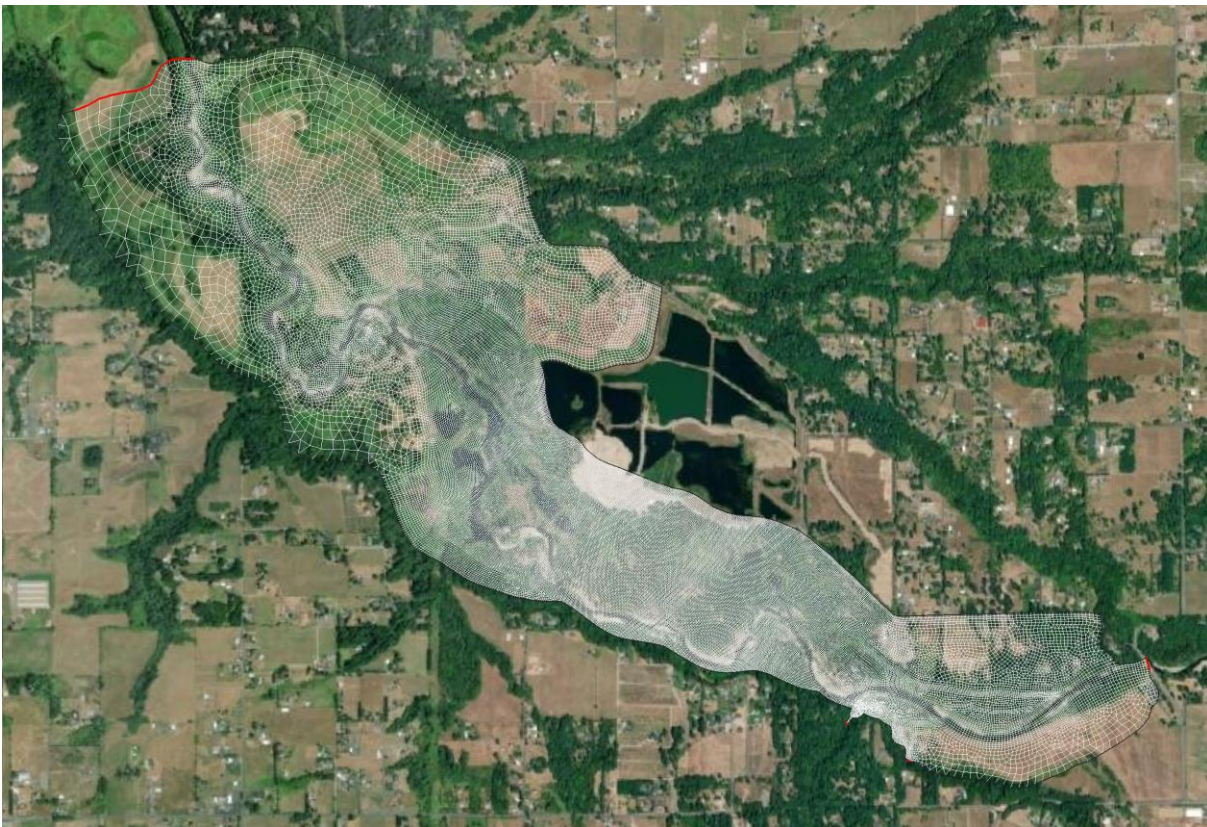
Figure 1. Hydrodynamic model grid, illustrating model extent and upstream/downstream boundary forcing locations.
