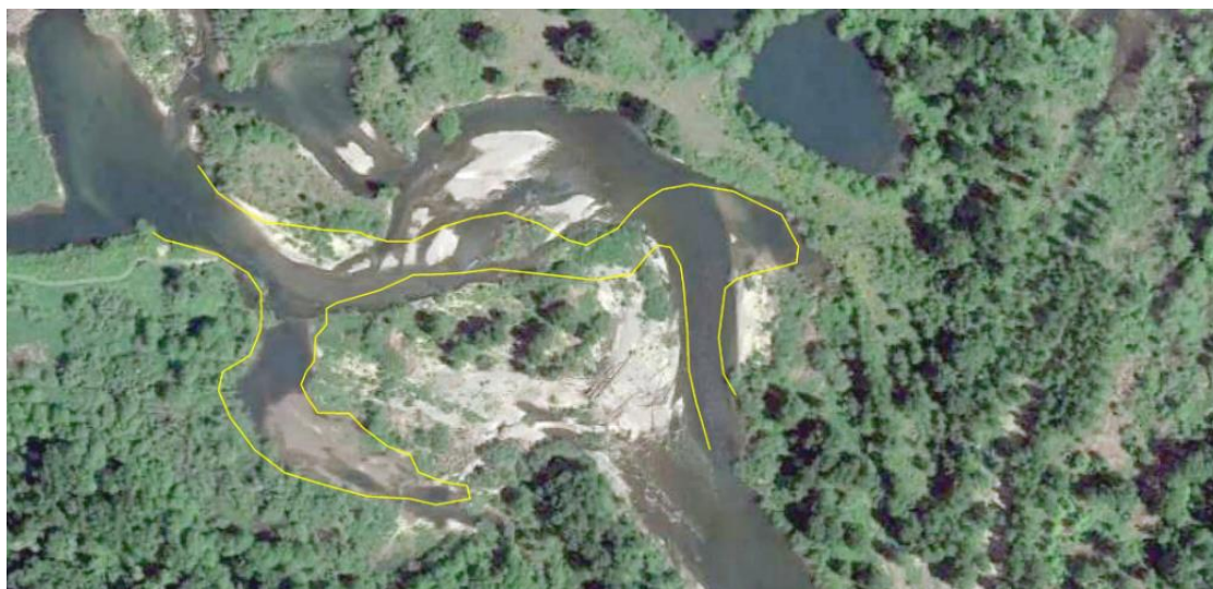
Figure 2. Change in river planform at river mile 8 between 2010 (indicated by the yellow line) and 2017 (shown in image).
